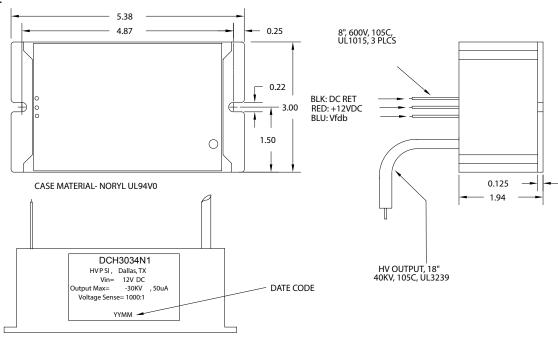
Operating Temperature: 0°C to +60°C (Case Temp., Full Load, Max Vo) Storage Temperature: -40°C to +85°C (Non-Operating, Case Temp.) Humidity: 0% to 95% (Non-Condensing) Altitude: 0 to 10,000 Ft (Standard Operating Conditions)
