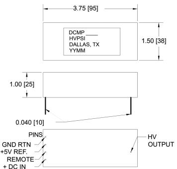
Operating Temperature: 0 to +60°C (Case Temp., Full Load, Max Vo) Storage Temperature: -40°C to +70°C (Non-Operating, Case Temp.) Humidity: 0% to 95% (Non-Condensing) Altitude: 0 to 10,000 Ft (Standard Operating Conditions)
